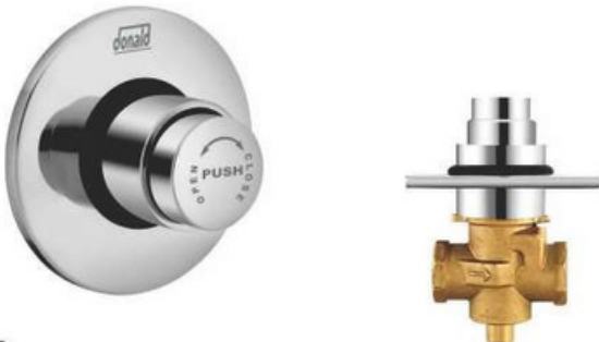
FVD-007 Flush Valve Dual Flow (25mm Size) Concealed Body with Round Plate in Brass (3.0/6.0 Liters per Flushing)
