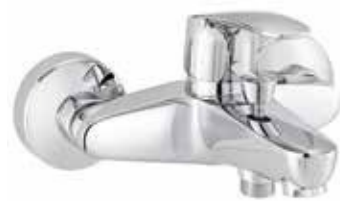
RAK17002 Single lever bath & shower mixer DN 15 without shower set ceramic cartridge-K35 aerator M 24 X 1 flow class CB automatic diverter: shower to bathtub shower outlet G 1/2" protected against back flow S- unions 1/2 X 3/4 inch European standard- EN 817
