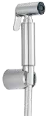
RAK32002 Brass Shattaf with supreme hose & wall bracket Connection 1/2 inch with supreme hose G1/2 x G 1/2 x 1200mm with wall bracket with dirt catching sieve
